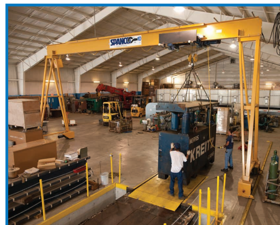
A 10-Ton Spanco PF Gantry Crane with power drive using guide angle for easy travel over a fixed route.
