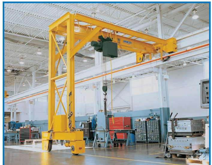
A Motorized 5-ton Spanco Wide-Flange Single-Leg Gantry Crane with an overall span of 20 feet and 15 feet under the beam.
