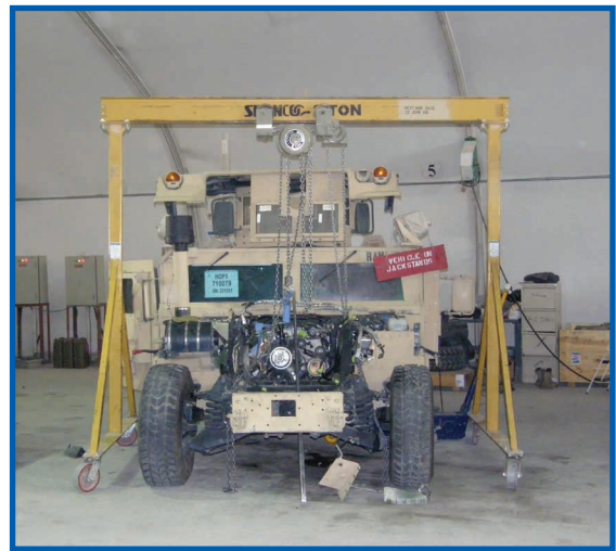
A Spanco E Series Fixed-Height Gantry Crane used for military vehicle maintenance in Afghanistan.
