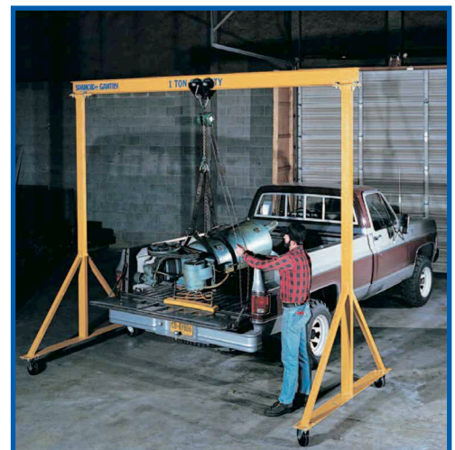
A 1-Ton Spanco E Series Gantry Crane lifting heavy parts from the back of a truck bed.
